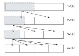
FIG. 2. Illustration of applying 3 successive temporal homogeneity transforms to an audio signal, by folding it twice ("2-fold"), three times ("3-fold") and four times ("4-fold"). The transform creates increasingly homogeneous signals by folding a reduced portion of the original signal. Note that the "1-fold" transform is the "identity" operator.
