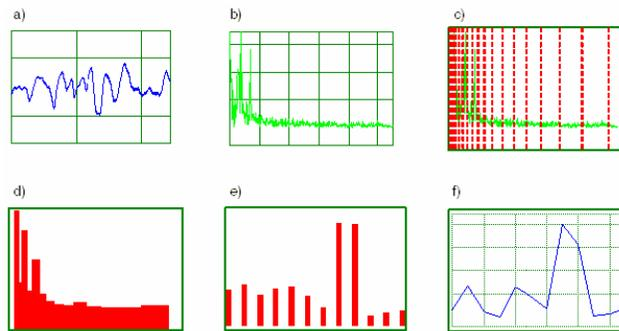
**Figure 2 - Steps to compute a PCP. The signal (a) is converted to Fast-Fourier representation (b); the FFT is divided into regions (c); the energy of each region is computed (d); these energies are folded into a 12-note vector (e); the final vector is normalized (f).**
